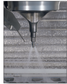
* Squirt Reamer (Retractable Reaming Tool) with Coolant through the Center (Rapid Attachment System).
